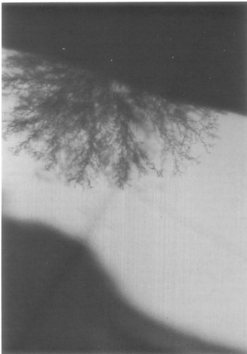
FIG. 11. Dendrite on Li anode (right; cathode is out of focus on left). Magnification 100 \times .
